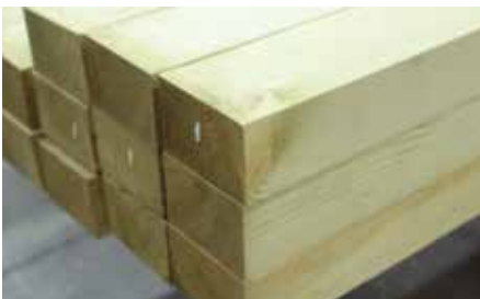
Impregnated substructure protects the wood against moisture and extends the service life
